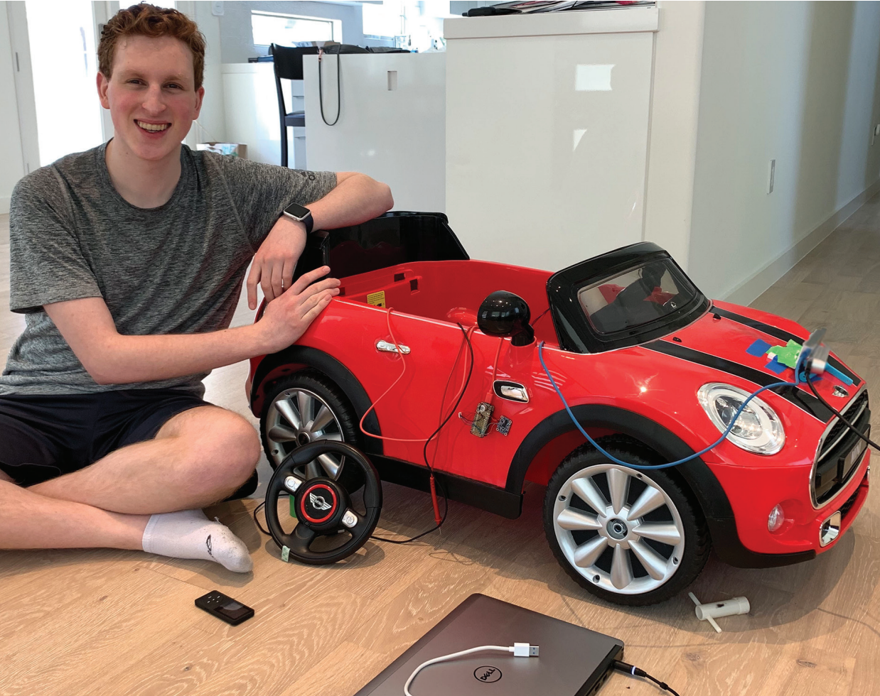
Ethan Saadia displays his self-driving car, a toy Mini Cooper modified with 3D printed parts and an electric control system.
