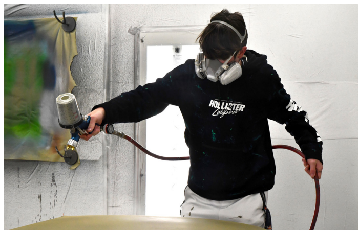
Taylor Keilman uses a spray gun to paint the hood of a car in the collision repair painting room. Photo by Rhian Davis.
