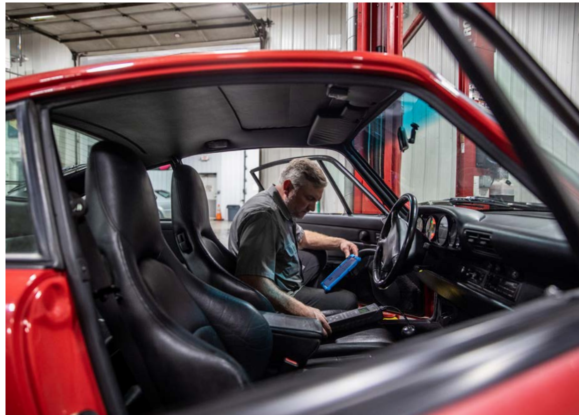
DIAGNOSIS / Zehr runs a diagnostics scanner on a Porsche for any fault codes that may be in the system. He has been a part of the family for over 8 years.
