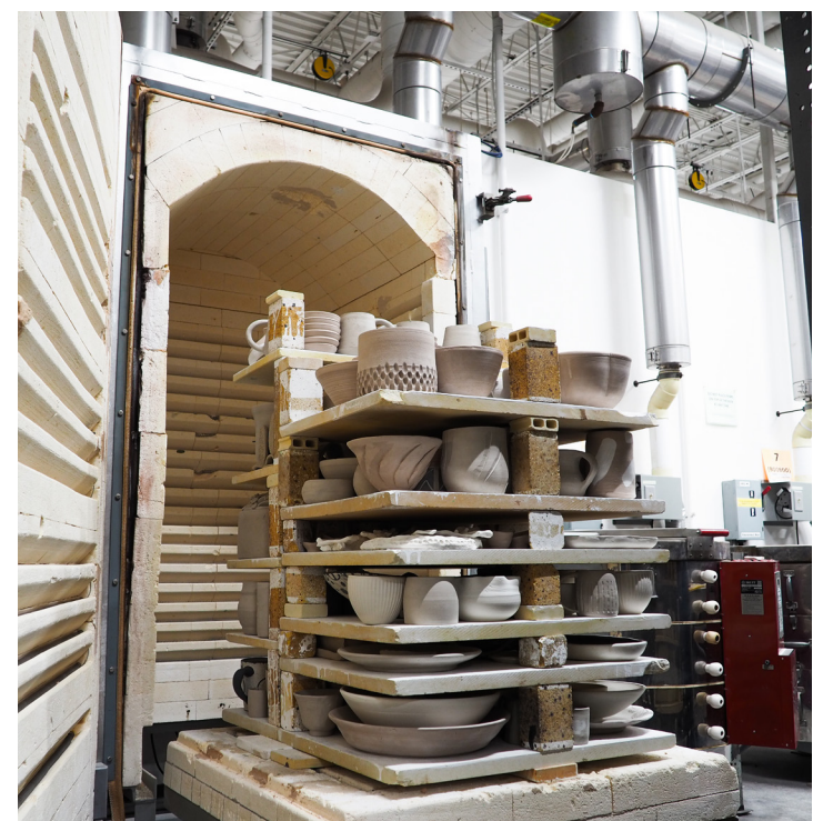
Ceramic ware must dry out before it is fired in a kiln. SÍLVIA CASACUBERTA PUIG — CRIMSON PHOTOGRAPHER
